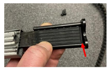
4 With the belt seated in the molded clamp, slide the molded clamp into the extrusion clamp and secure with two screws.
